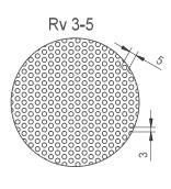
The exemplary supply air wall unit with a window  $QAW-5920 \times 2300 \times 750$  (cover image) shown here consists of 10 assembled individual elements. A nozzle panel with adjustable SEV elements for homogeneous air distribution is located behind the perforated front panel. The front panel has a perforation pattern of Rv 3-5. Furthermore, optional blind panels can be installed in the wall, ceiling or floor areas.
